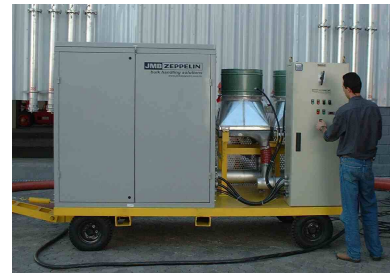
AGU – Air Generation Unit
